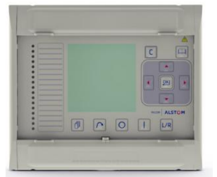
Figure 2 MiCOM C264 front view (40TE variant)
