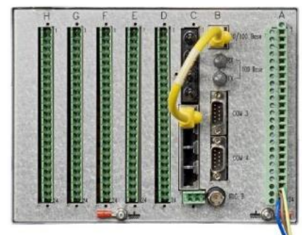
Figure 5 MiCOM Alstom C264 rear view (40TE variant)
